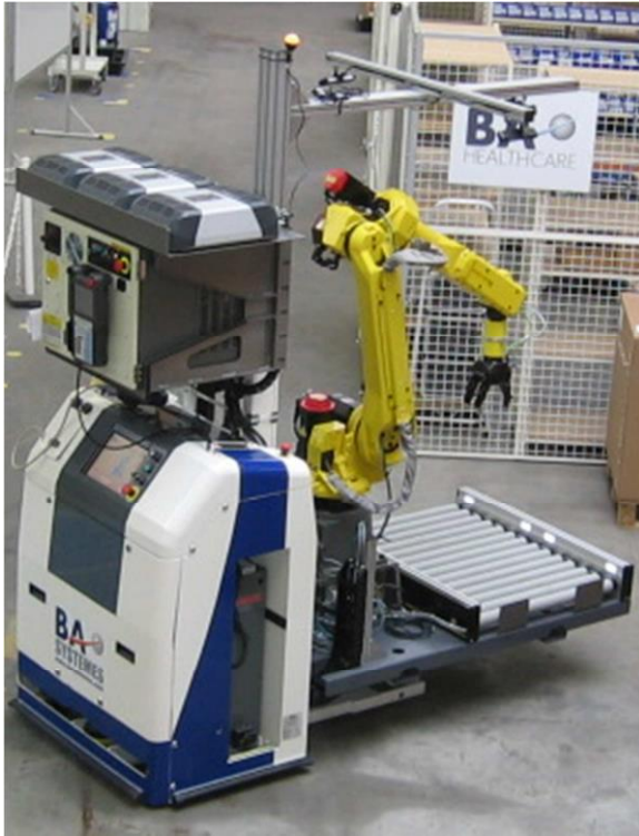
Figure 1. The autonomous robot composed of a mobile platform, industrial robotic arm, and a three finger gripper.
